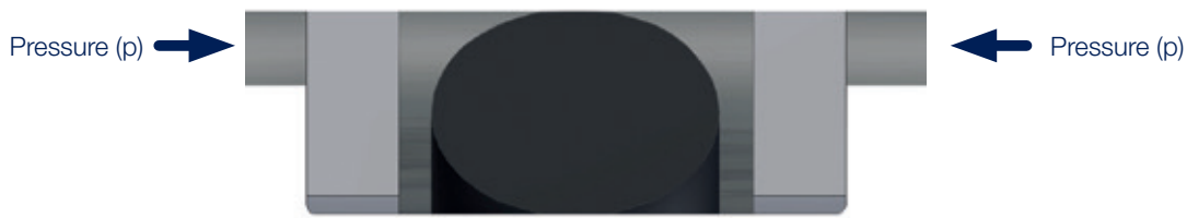
Figure 2: Double-acting O-ring with 2 back-up rings
