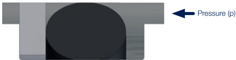
Figure 1: Single-acting O-ring with 1 back-up ring
